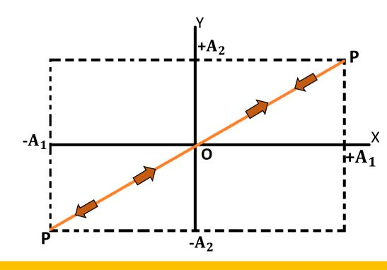
Equation (4) represents a pair of coincident straight lines passing through the origin with a slope of  $\frac{A_2}{A_1}$  as shown in the figure.
